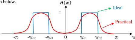
Band stop filter allows entire band of frequency signals over the range  $-\pi \le w \le -wc_2 \& -wc_1 \le w \le wc_1 \& wc_2 \le w \le \pi$  except unwanted band of frequency signals. Ideal and practical characteristics of a band stop filter as shown below.
