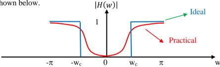
Band pass filter allows only a certain band of frequency signals over the range  $-w_{C2} \le w \le -w_{C1}$  and attenuate all other frequency signals. Ideal and practical characteristics of a band pass filter as shown below.
